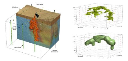
Figure: Left: Model, with source/detector locations; Right top: truth; Bottom: a PaLS joint reconstruction.
